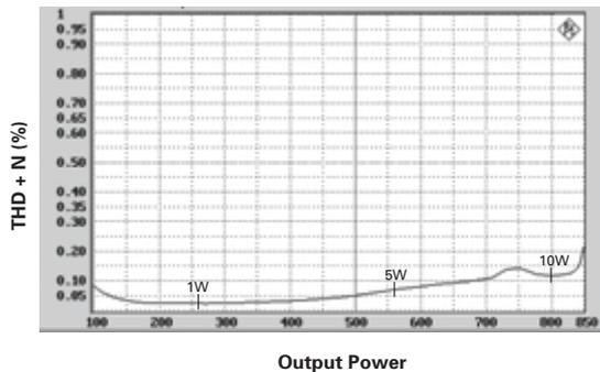
The plot shows Distortion v Power into an 8 $\Omega$  load at 1kHz. This plot clearly demonstrates the unequalled performance of the Zetex solution. Typical distortion of 0.05% at 1W can be seen with better than 0.15% at 10W. Truly world class performance.
