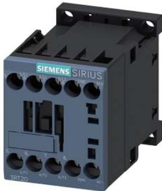
power contactor, AC-3 7 A, 3 kW / 400 V 1 NC, 24 V DC 0.7-1.25\* US, suppressor diode integrated, 3-pole, size S00, screw terminal suitable for PLC outputs not expandable with auxiliary switch
