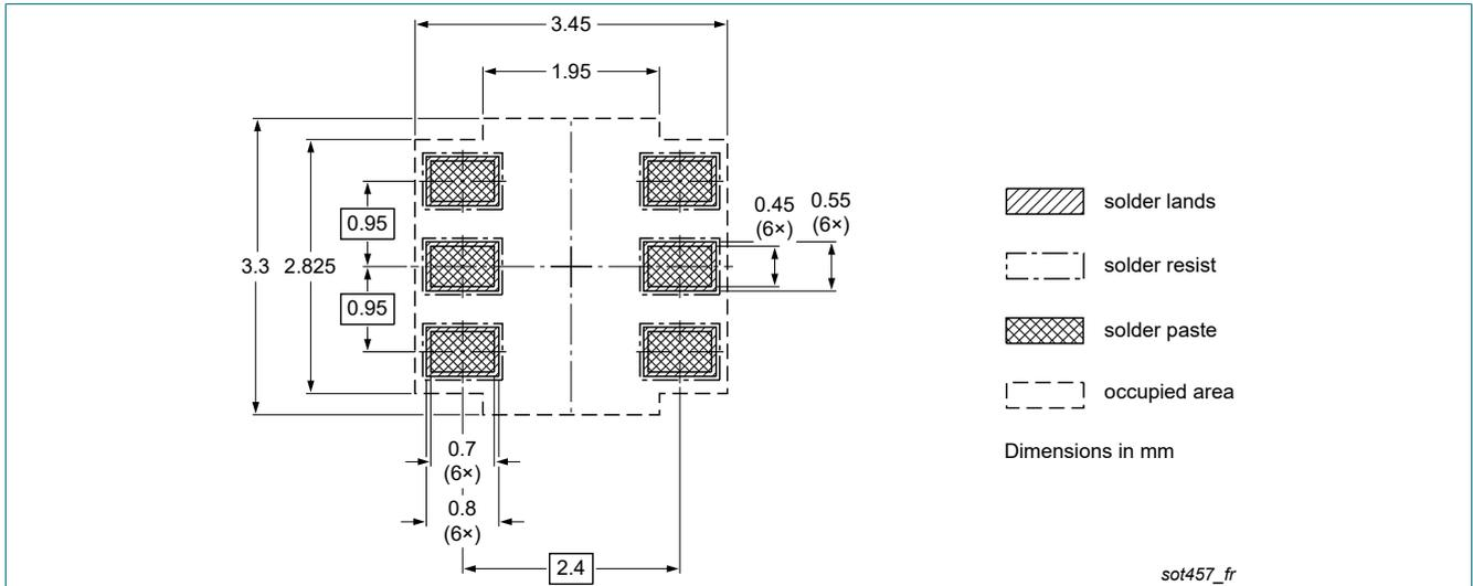
Fig. 6. Reflow soldering footprint for SC-74; TSOP6 (SOT457)
