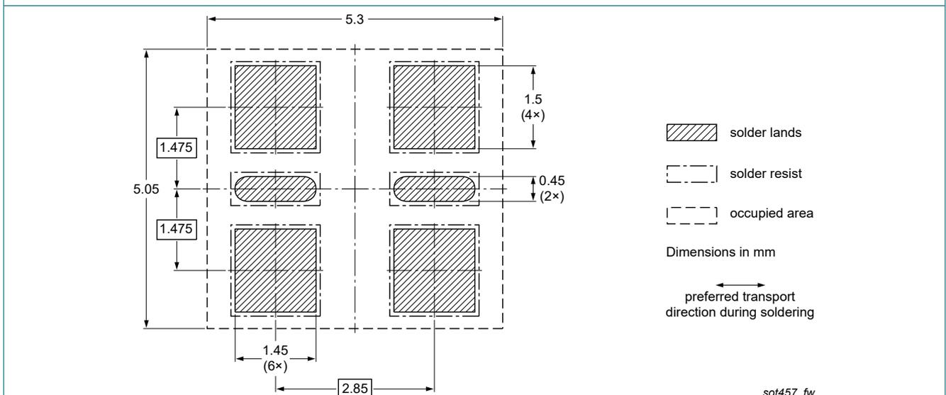
Fig. 7. Wave soldering footprint for SC-74; TSOP6 (SOT457)
