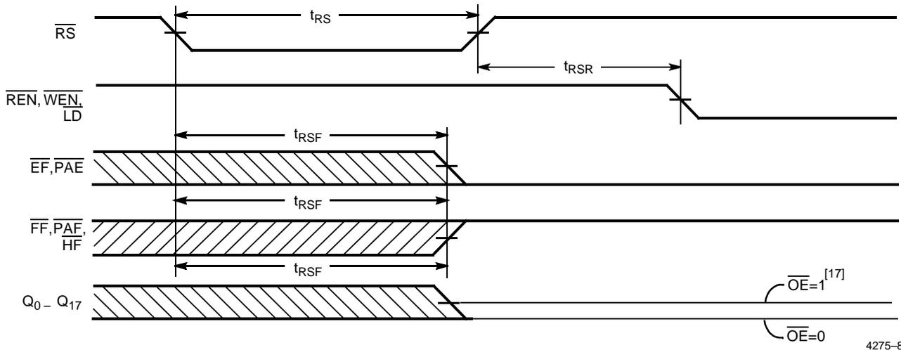
**First Data Word Latency after Reset with Simultaneous Read and Write**
