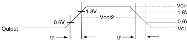
Output Test Conditions for  $V_{CC} = 2.5V \pm 5\%$
