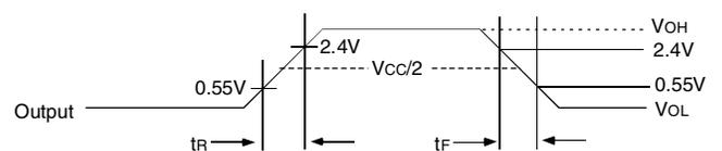
Output Test Conditions for  $V_{CC} = 3.3V \pm 5\%$
