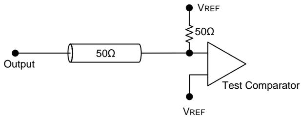
(b)  $t_{CHQZ}$  and  $t_{CHQX1}$  are specified with 5pF load capacitance and measured when transition occurs  $\pm 100\text{mV}$  from the steady state voltage.
