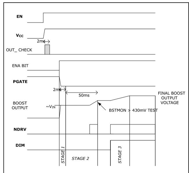
Figure 3. Boost Startup (I<sup>2</sup>C Operation)
