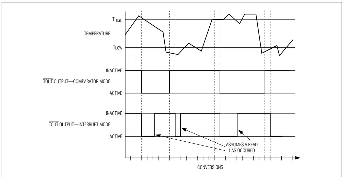
Figure 6.  $\overline{\text{TOUT}}$  Operation Example
