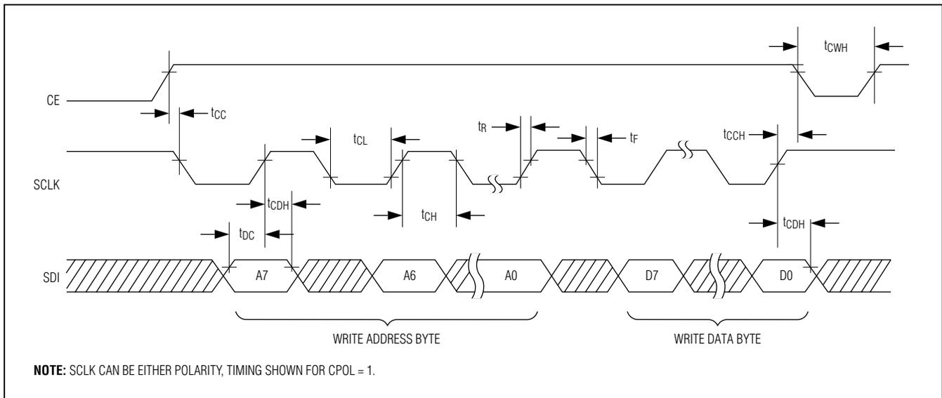
Figure 4. Timing Diagram: SPI Write Data Transfer
