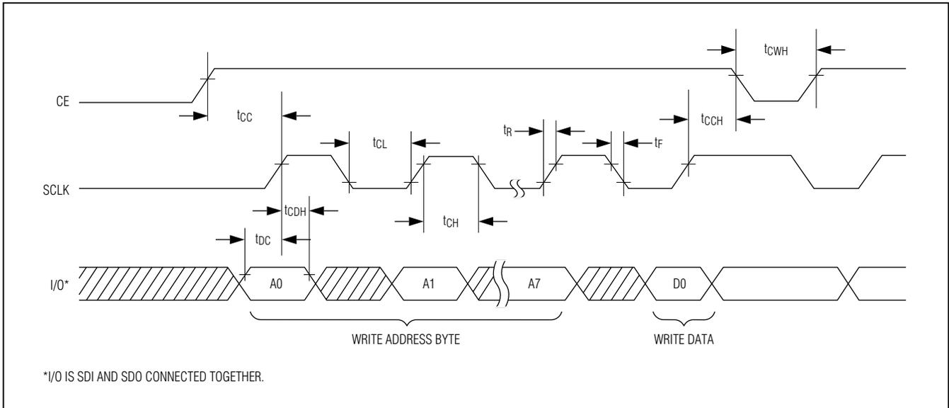
Figure 2. Timing Diagram: 3-Wire Write Data Transfer
