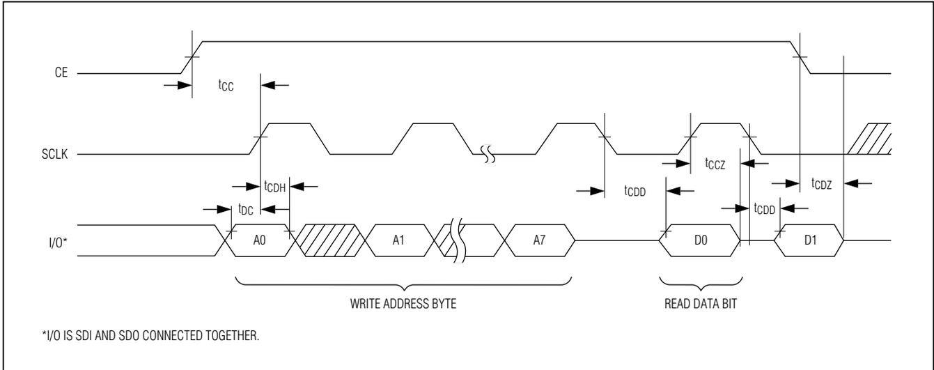
Figure 1. Timing Diagram: 3-Wire Read Data Transfer
