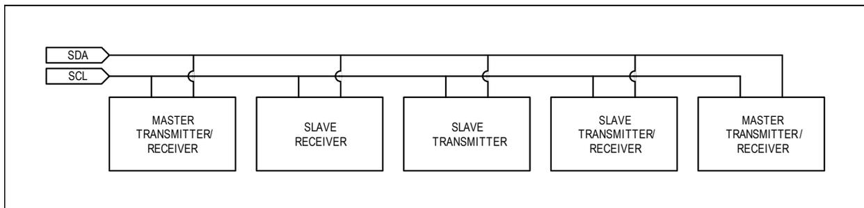
Figure 2. I<sup>2</sup>C system configuration.
