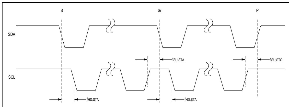
Figure 3. I<sup>2</sup>C START and STOP conditions.
