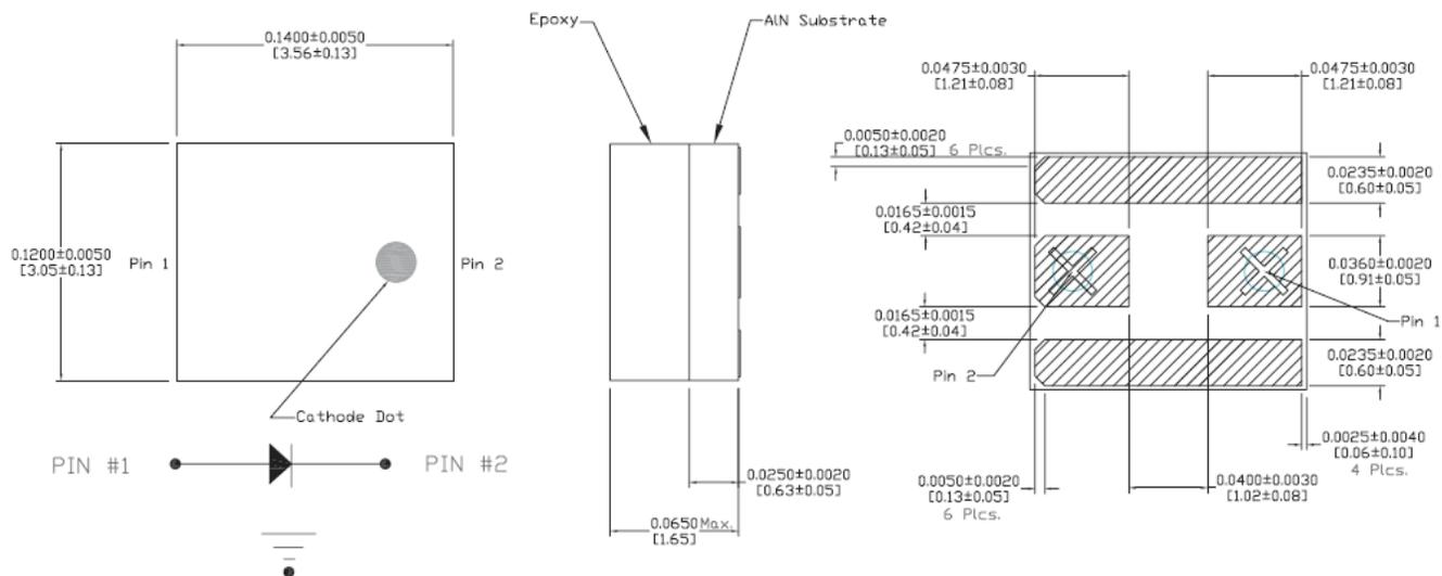
Pin function for Silicon PIN diode.
