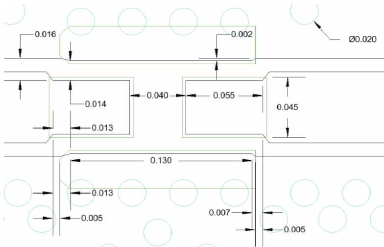
Plated through, filled and plated over vias
