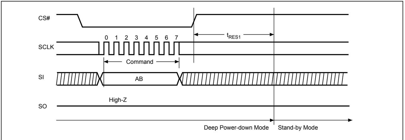
**Figure 27. Read Electronic Manufacturer & Device ID (REMS) Sequence (Command 90 or EF or DF)**
