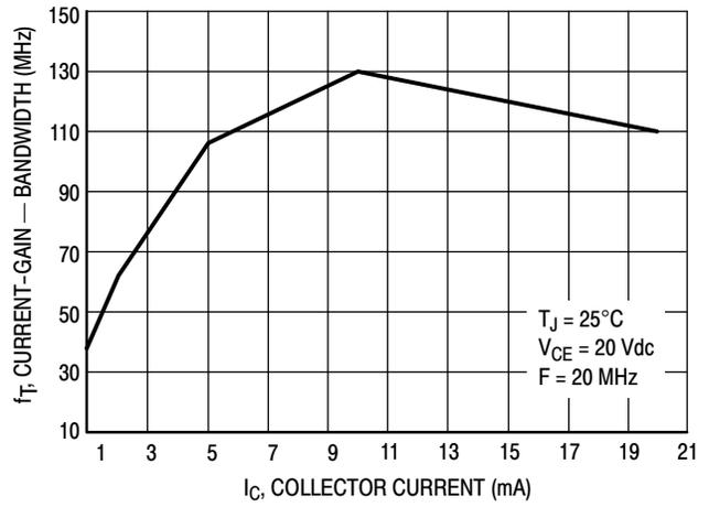
Figure 3. Current-Gain - Bandwidth
