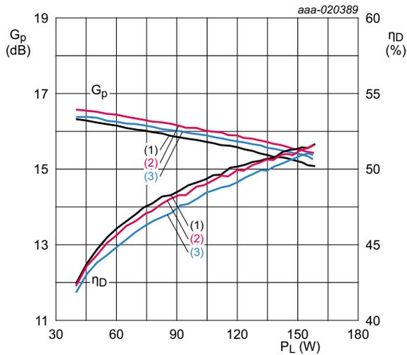
$V_{DS} = 28\text{ V}; I_{Dq} = 400\text{ mA (main device)}; V_{GS(amp)peak} = 0.5\text{ V}.$
