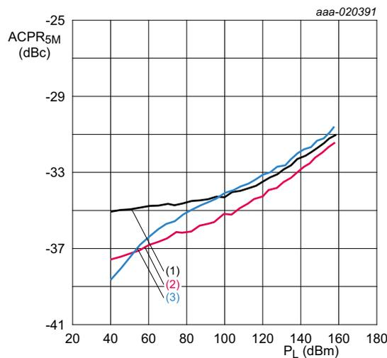
$V_{DS} = 28\text{ V}; I_{Dq} = 400\text{ mA (main device)}; V_{GS(amp)peak} = 0.5\text{ V}.$
