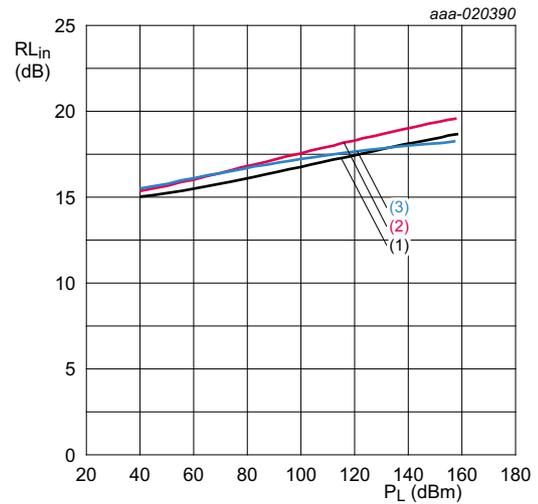
$V_{DS} = 28\text{ V}; I_{Dq} = 400\text{ mA (main device)}; V_{GS(amp)peak} = 0.5\text{ V}.$
