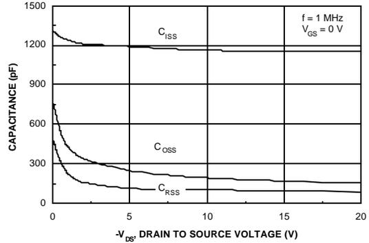
Figure 8. Capacitance Characteristics.
