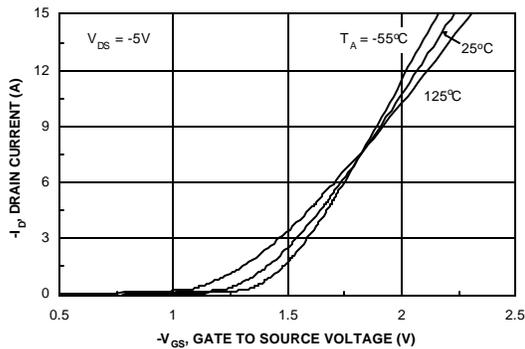
Figure 5. Transfer Characteristics.
