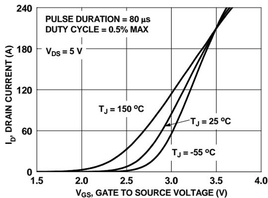
**Figure 5. Transfer Characteristics**
