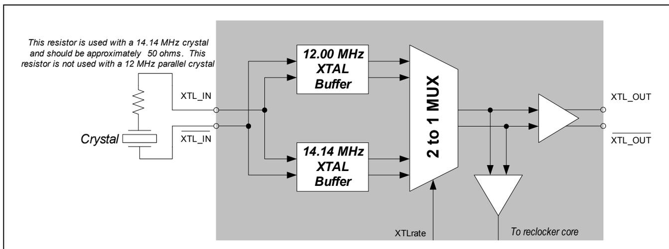
The series resonant crystal should operate at 14.14 MHz with a frequency stability of +/- 50 ppm or better, equivalent series resistance of 80Ω or less, drive level of < 0.2 mW, and static capacitance of less than 5.0 pF. The parallel resonant crystal should operate at 12.00 MHz with a frequency stability of +/- 50 ppm or better, equivalent series resistance of 80Ω or less, drive level of < 0.2 mW, and static capacitance of less than 5.0 pF.
