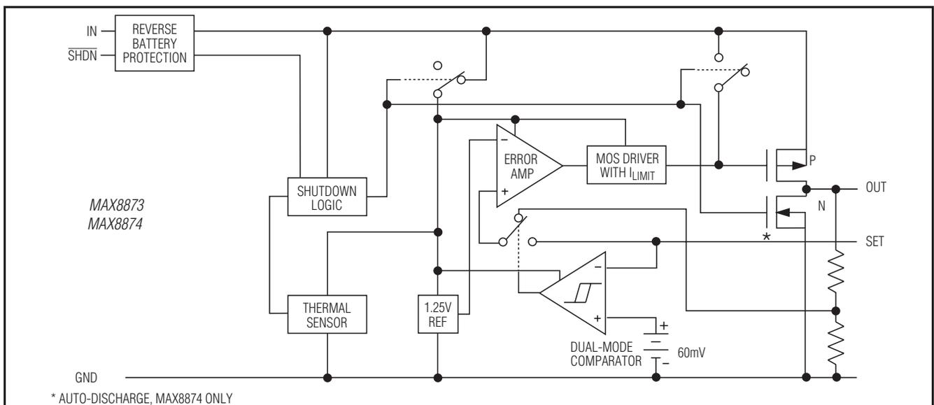
Figure 1. Functional Diagram
