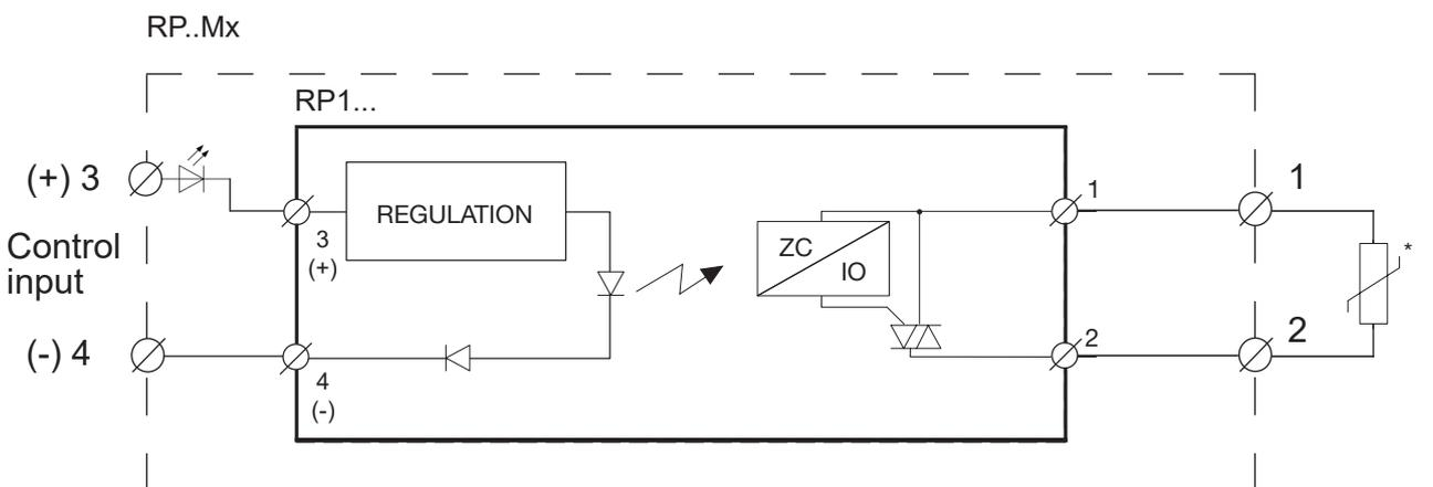
\* The varistor is not included in the solid state relay. Connecting a varistor across terminals 1-2 helps protect the solid state relay against damages by over-voltage
