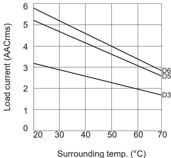
Derating curve is used for finding max. load current at an elevated ambient temperature. The 3 lines in the graph represent the 3 nominal current ratings of the RP1 series (RP1...D3/D5/D6). When used at full load current, the relays must be placed vertically. If more than one relay is mounted, please allow a minimum distance of 20 mm in between for sufficient air cooling.
