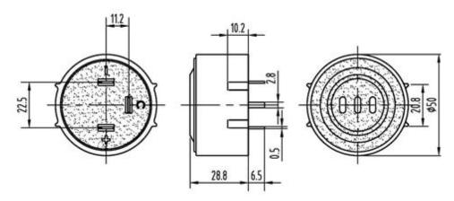
Only when apply  $12V_{\mbox{\scriptsize DC}}$  on pin "c",the product can produce sound
