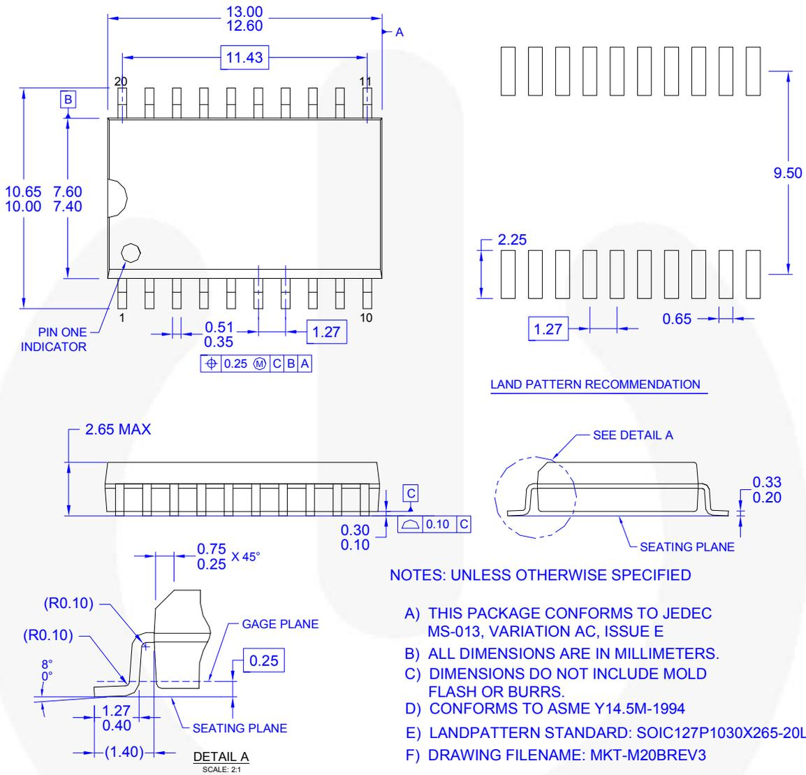
**Figure 57. 20-Pin, Small Outline Integrated Circuit (SOIC) Package**
