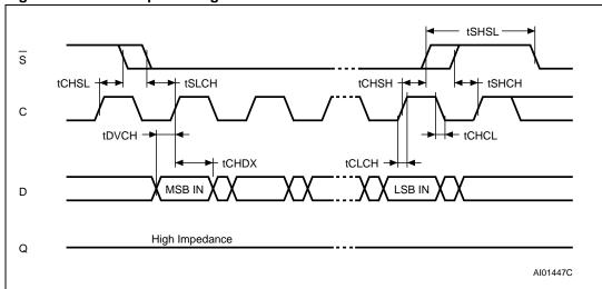
Figure 21. Write protect setup and hold timing during WRSR when SRWD =1
