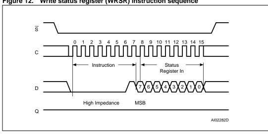
Figure 12. Write status register (WRSR) instruction sequence
