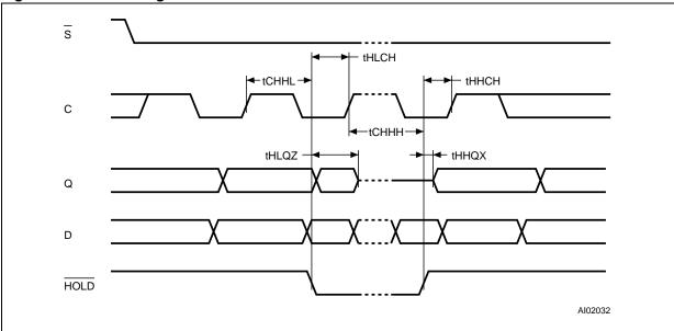
Figure 23. Output timing
