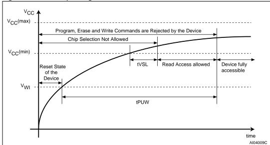
Figure 18. Power-up timing
