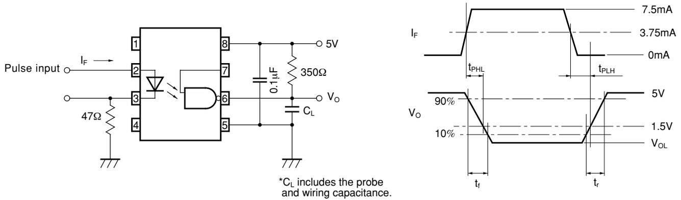
**Fig.2 Test Circuit for Enable Propagation Delay Time**
