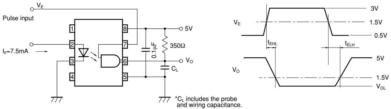
**Fig.3 Test Circuit for Instantaneous Common Mode Rejection Voltage**
