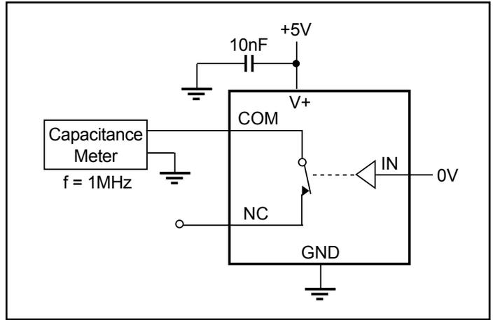
Figure 6. Channel-On Capacitance
