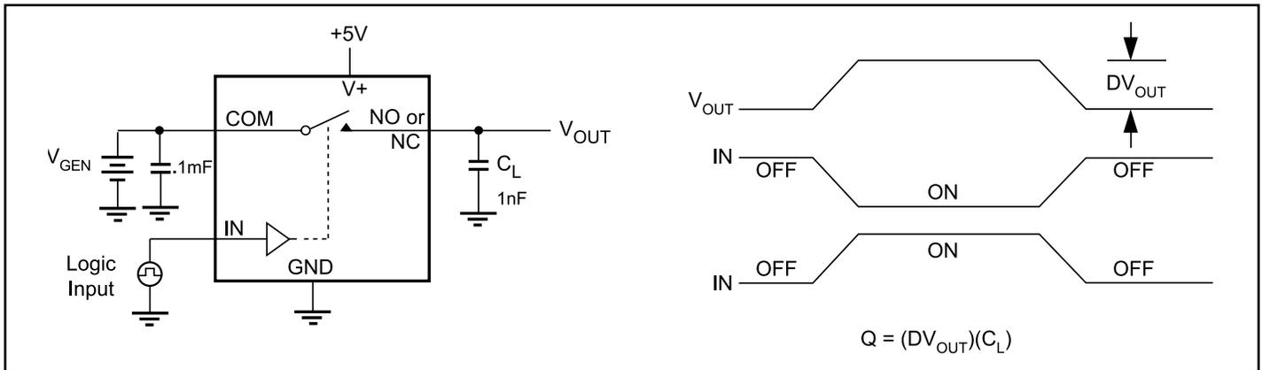
Figure 2. Charge Injection
