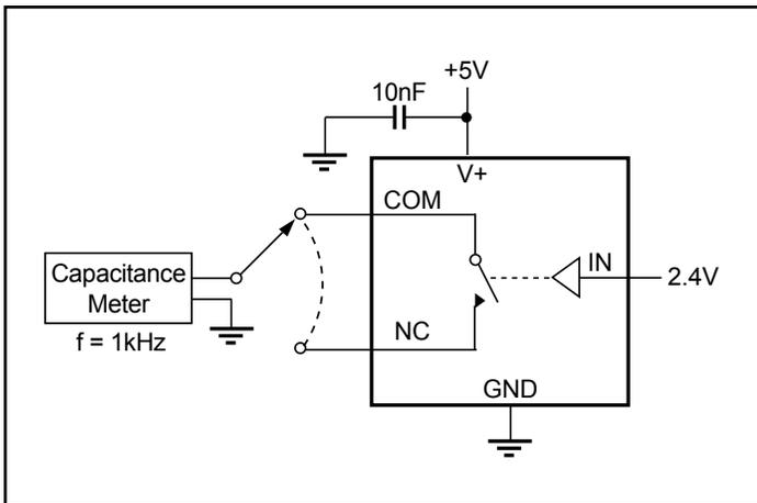
Figure 5. Channel-Off Capacitance
