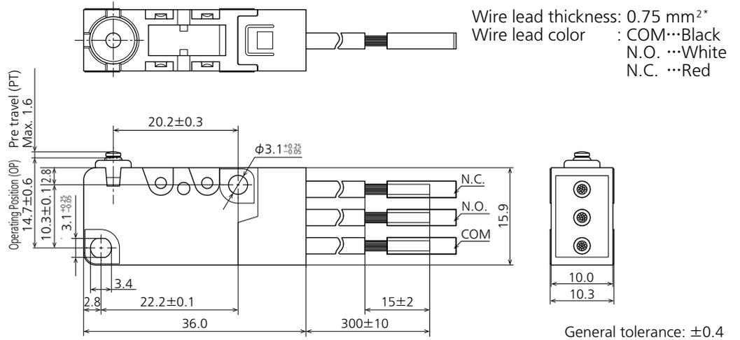
Note) Dimensions of the actuator types are the same as those of corresponding solder and .187 quick-connect terminal types.
