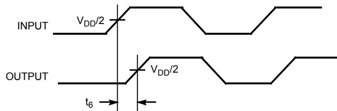
Figure 9. Device-Device Skew
