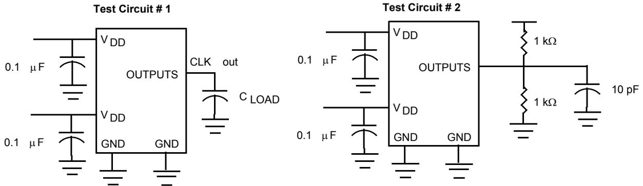
For parameter  $t_g$  (output slew rate) on -1H devices
