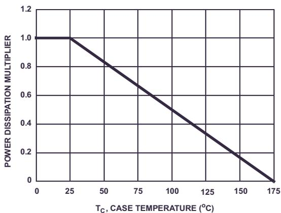
**Figure 1. Normalized Power Dissipation vs Ambient Temperature**
