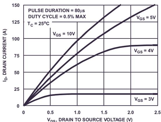
**Figure 8. Saturation Characteristics**
