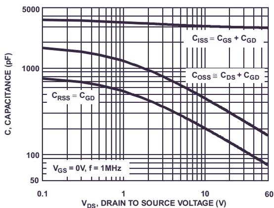
**Figure 13. Capacitance vs Drain to Source Voltage**
