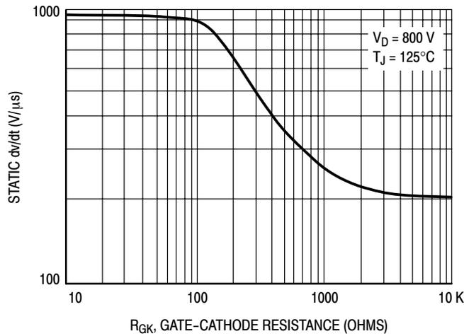
Figure 9. Exponential Static dv/dt versus Gate-Cathode Resistance
