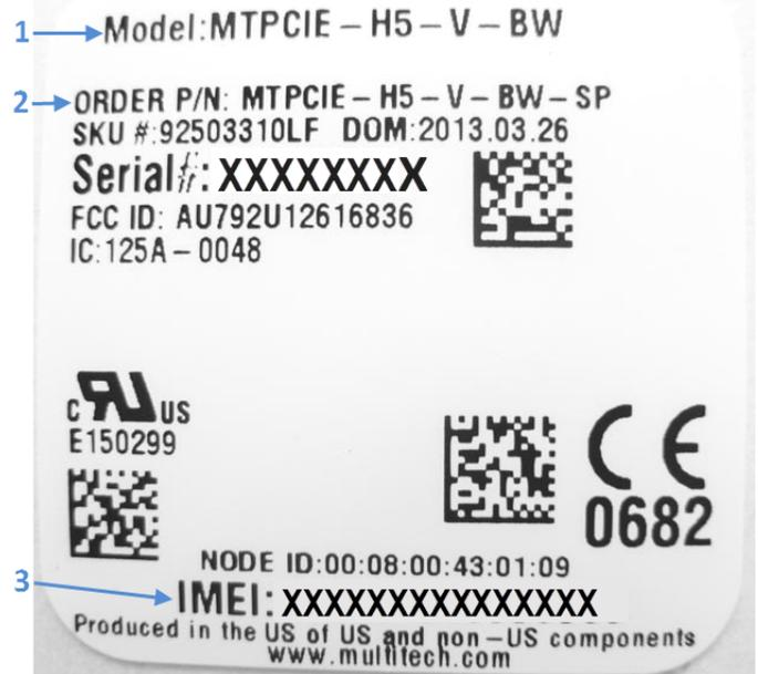
Labels are positioned on the device as follows:
