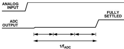
Figure 38. Sinc<sup>3</sup> Zero Latency Operation
