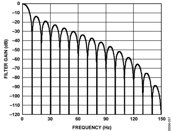
Figure 58. Filter Response for Average + Decimate Filter (Sinc<sup>4</sup> Filter, FS[9:0] = 30, Average by 16)
