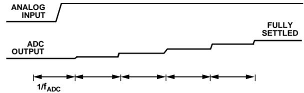
Figure 29. Asynchronous Step Change in Analog Input
