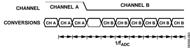
Figure 61. Fast Settling, Sinc<sup>3</sup> Filter
