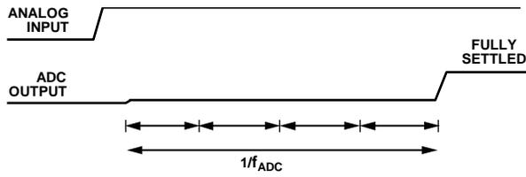
Figure 30. Sinc<sup>4</sup> Zero Latency Operation
