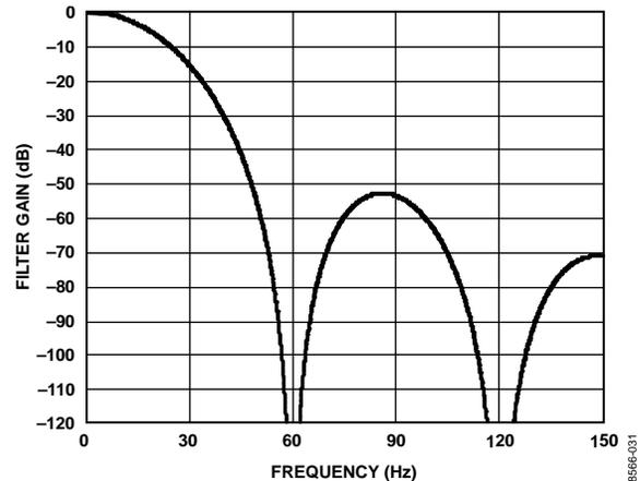
Figure 32. Sinc<sup>4</sup> Filter Response (FS[9:0] = 80)
