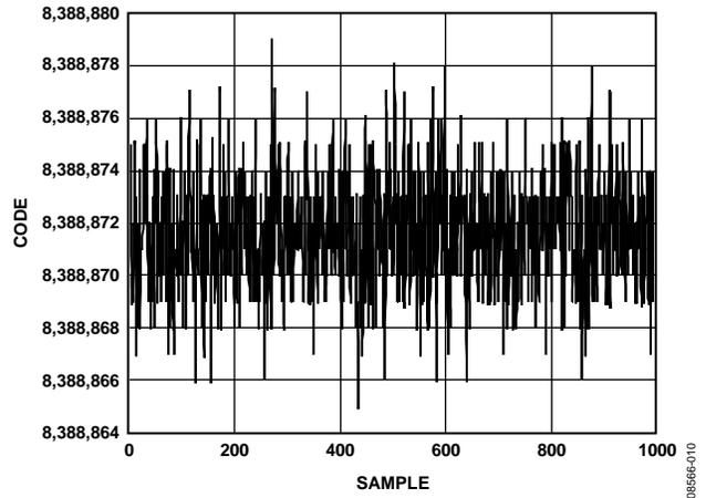
Figure 10. Noise ( $V_{REF} = AV_{DD} = 5\text{ V}$ , Output Data Rate = 42.1 Hz (FS[9:0] = 6, Average by 16), Gain = 1, Chop Disabled, Sinc<sup>4</sup> Filter)
