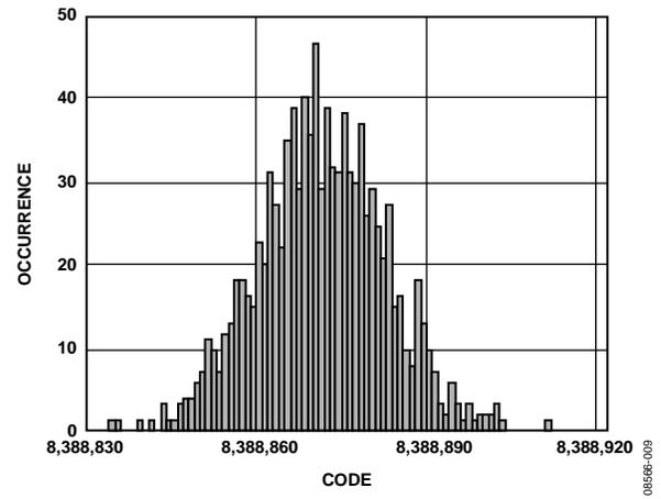
Figure 9. Noise Distribution Histogram ( $V_{REF} = AV_{DD} = 5\text{ V}$ , Output Data Rate = 2400 Hz, Gain = 1, Chop Disabled, Sinc<sup>4</sup> Filter)
