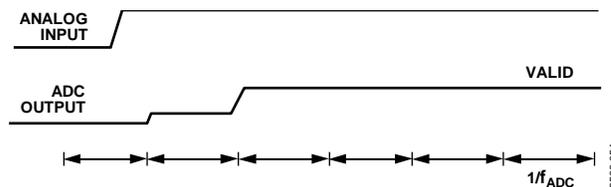
Figure 55. Step Change on Analog Input,  $\text{Sinc}^4$  Filter
