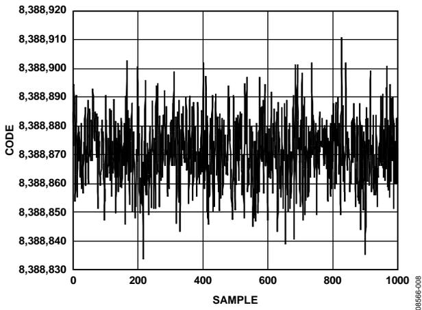
Figure 8. Noise ( $V_{REF} = AV_{DD} = 5\text{ V}$ , Output Data Rate = 2400 Hz, Gain = 1, Chop Disabled, Sinc<sup>4</sup> Filter)
