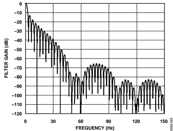
Figure 66. Filter Response for Average + Decimate Filter (Sinc<sup>3</sup> Filter, FS[9:0] = 96, Average by 16)
