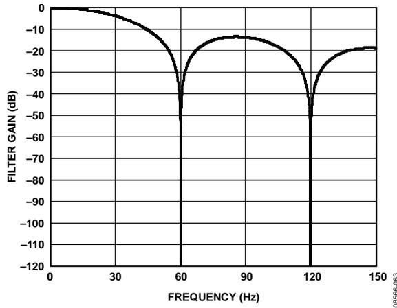
Figure 64. Filter Response for Average + Decimate Filter (Sinc<sup>3</sup> Filter, FS[9:0] = 5, Average by 16)
