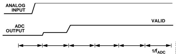
Figure 62. Step Change on Analog Input, Sinc<sup>3</sup> Filter
