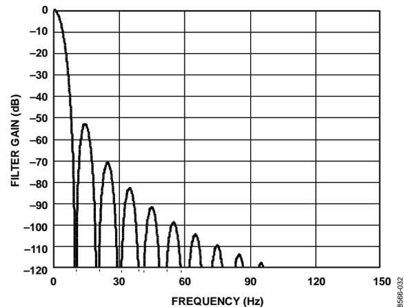
Figure 33. Sinc<sup>4</sup> Filter Response (FS[9:0] = 480)
