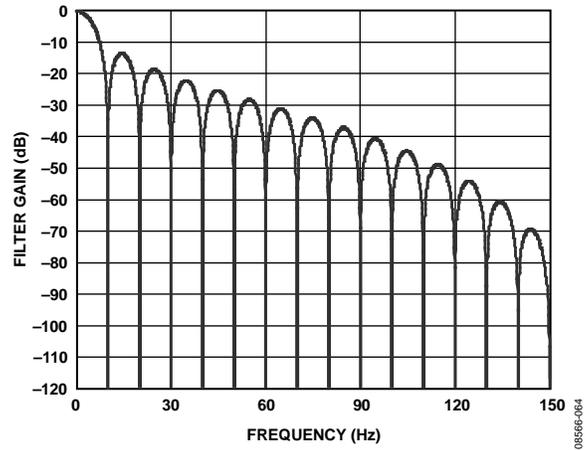
Figure 65. Filter Response for Average + Decimate Filter (Sinc<sup>3</sup> Filter, FS[9:0] = 30, Average by 16)
