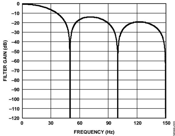
Figure 56. Filter Response for Average + Decimate Filter (Sinc<sup>4</sup> Filter, FS[9:0] = 6, Average by 16)
