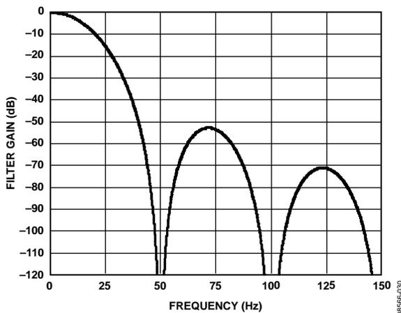
Figure 31. Sinc<sup>4</sup> Filter Response (FS[9:0] = 96)
