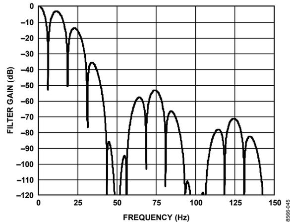
Figure 46.  $Sinc^4$  Filter Response ( $FS[9:0] = 96$ , Chop Enabled)
