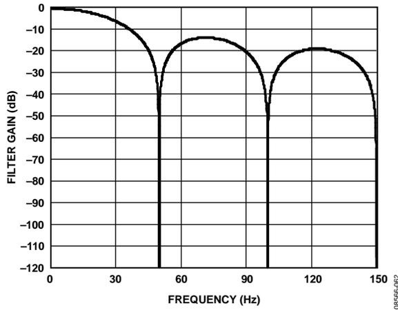
Figure 63. Filter Response for Average + Decimate Filter (Sinc<sup>3</sup> Filter, FS[9:0] = 6, Average by 16)
