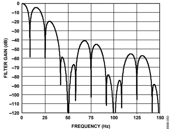
Figure 51. Sinc<sup>3</sup> Filter Response ( $FS[9:0] = 96$ , Chop Enabled)
