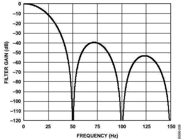
Figure 39. Sinc<sup>3</sup> Filter Response (FS[9:0] = 96)
