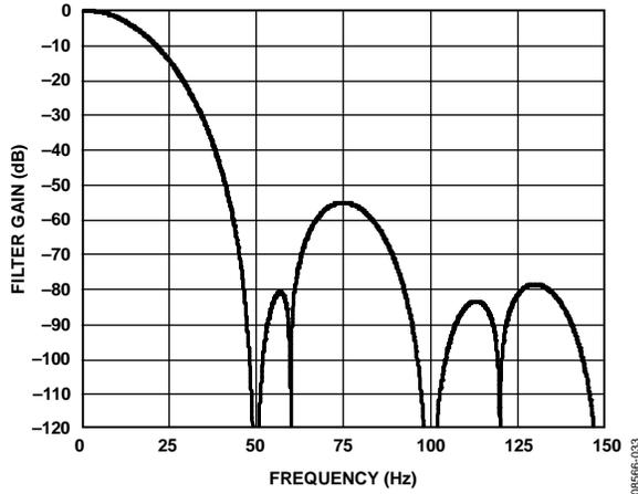
Figure 34. Sinc<sup>4</sup> Filter Response (FS[9:0] = 96, REJ60 = 1)
