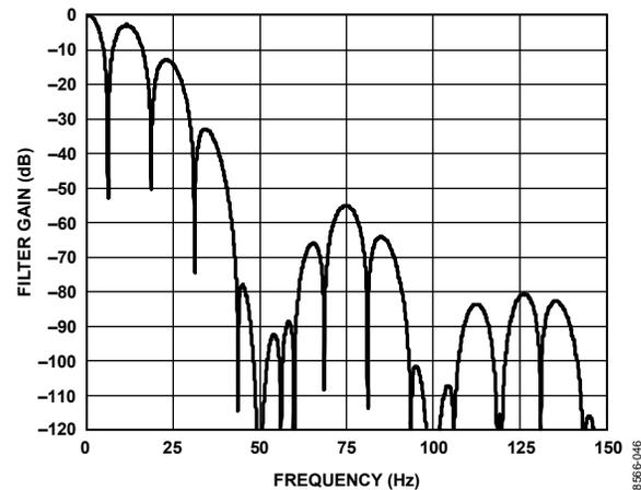
Figure 47.  $Sinc^4$  Filter Response ( $FS[9:0] = 96$ , Chop Enabled,  $REJ60 = 1$ )
