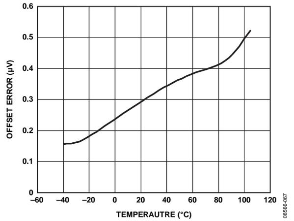
Figure 15. Offset vs. Temperature (Gain = 128, Chop Disabled)
