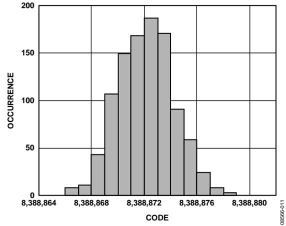
Figure 11. Noise Distribution Histogram ( $V_{REF} = AV_{DD} = 5\text{ V}$ , Output Data Rate = 42.1 Hz (FS[9:0] = 6, Average by 16), Gain = 1, Chop Disabled, Sinc<sup>4</sup> Filter)
