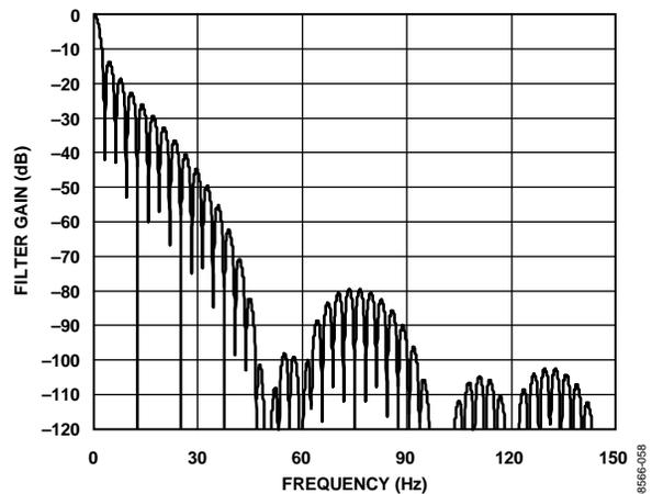
Figure 59. Filter Response for Average + Decimate Filter (Sinc<sup>4</sup> Filter, FS[9:0] = 96, Average by 16)
