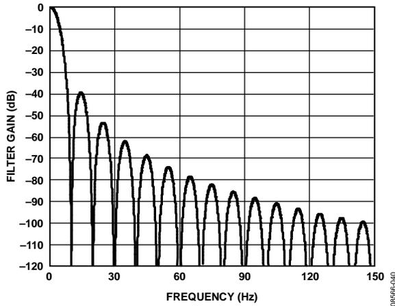
Figure 41. Sinc<sup>3</sup> Filter Response (FS[9:0] = 480)
