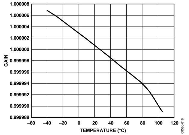
Figure 16. Gain vs. Temperature (Gain = 1)
