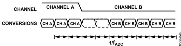
Figure 49. Channel Change (Sinc<sup>3</sup> Chop Enable)
