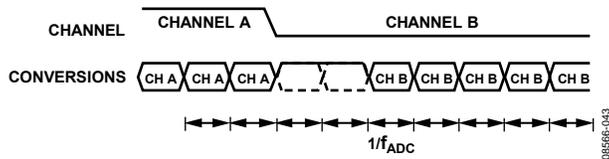
Figure 44. Channel Change ( $Sinc^4$  Chop Enabled)
