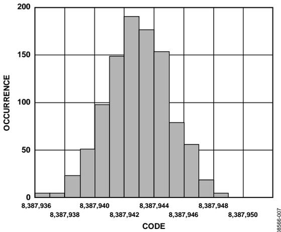
Figure 7. Noise Distribution Histogram ( $V_{REF} = AV_{DD} = 5\text{ V}$ , Output Data Rate = 4.7 Hz, Gain = 128, Chop Disabled, Sinc<sup>4</sup> Filter)
