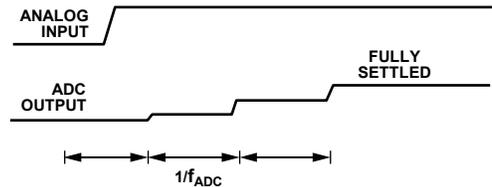
Figure 50. Asynchronous Step Change in Analog Input (Sinc<sup>3</sup> Chop Enabled)
