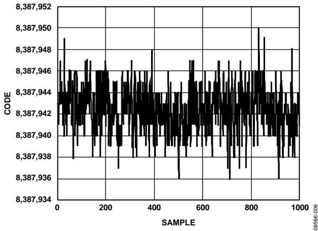
Figure 6. Noise ( $V_{REF} = AV_{DD} = 5\text{ V}$ , Output Data Rate = 4.7 Hz, Gain = 128, Chop Disabled, Sinc<sup>4</sup> Filter)
