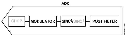
Figure 60. Fast Settling Mode, Sinc<sup>3</sup> Filter
