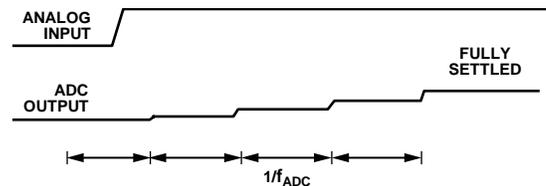
Figure 37. Asynchronous Step Change in Analog Input
