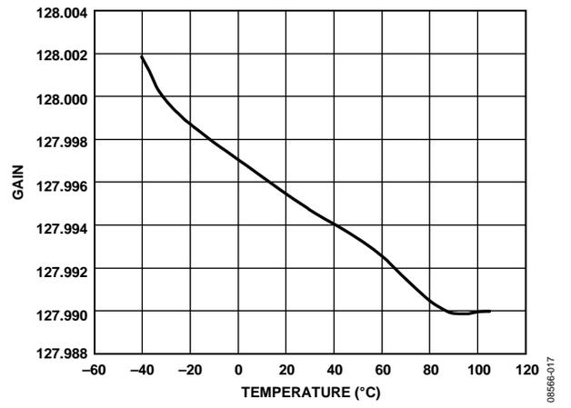
Figure 17. Gain vs. Temperature (Gain = 128)
