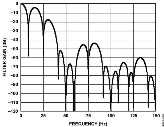
Figure 52.  $\text{Sinc}^3$  Filter Response
