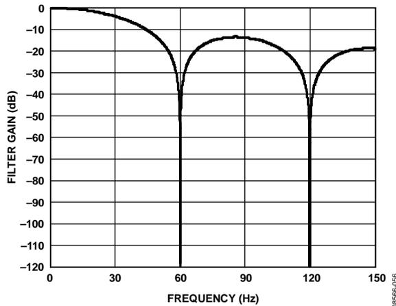
Figure 57. Filter Response for Average + Decimate Filter (Sinc<sup>4</sup> Filter, FS[9:0] = 5, Average by 16)
