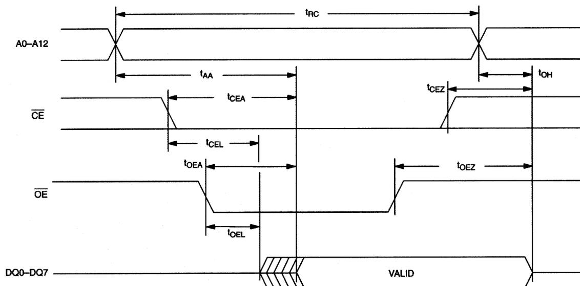
**READ CYCLE, AC CHARACTERISTICS** $(V_{CC} = 5.0V \pm 10\%)$
