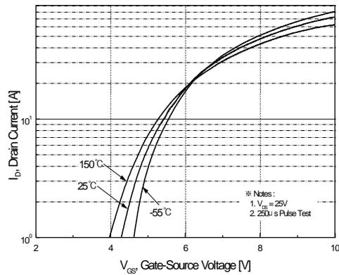
**Figure 2. Transfer Characteristics**
