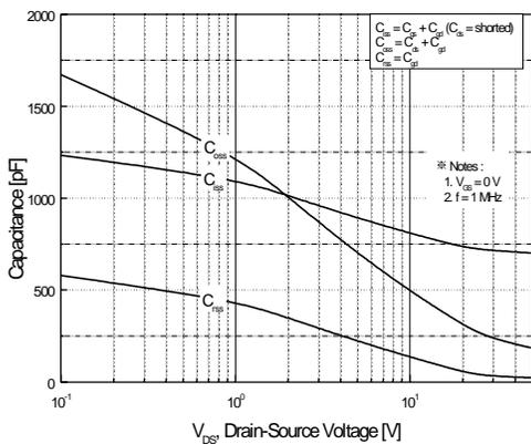
**Figure 5. Capacitance Characteristics**
