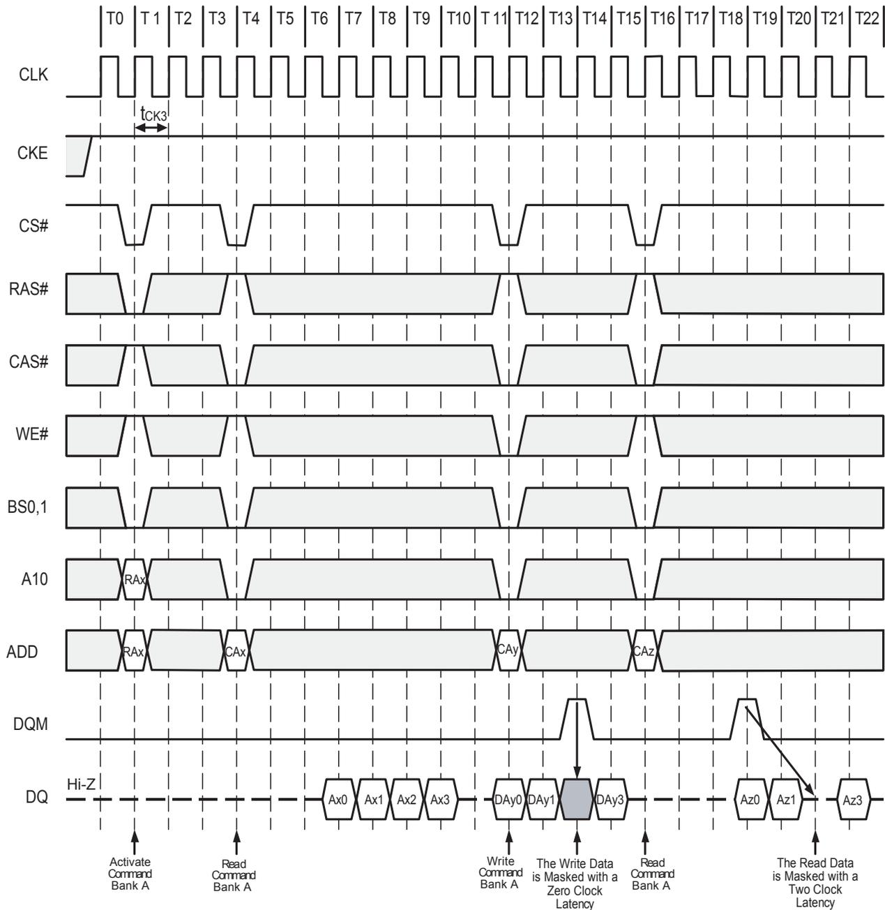
Interleaving Column Read Cycle (Burst Length=4,CAS#Latency=2)
