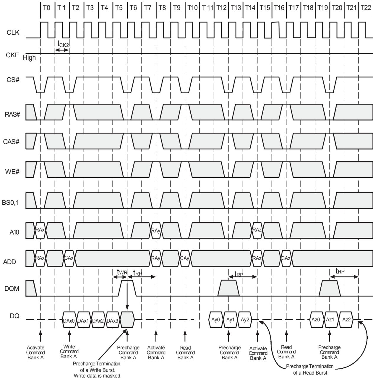
**Precharge Termination of a Burst (Burst Length=4,8 or Full Page,CAS#Latency=3)**
