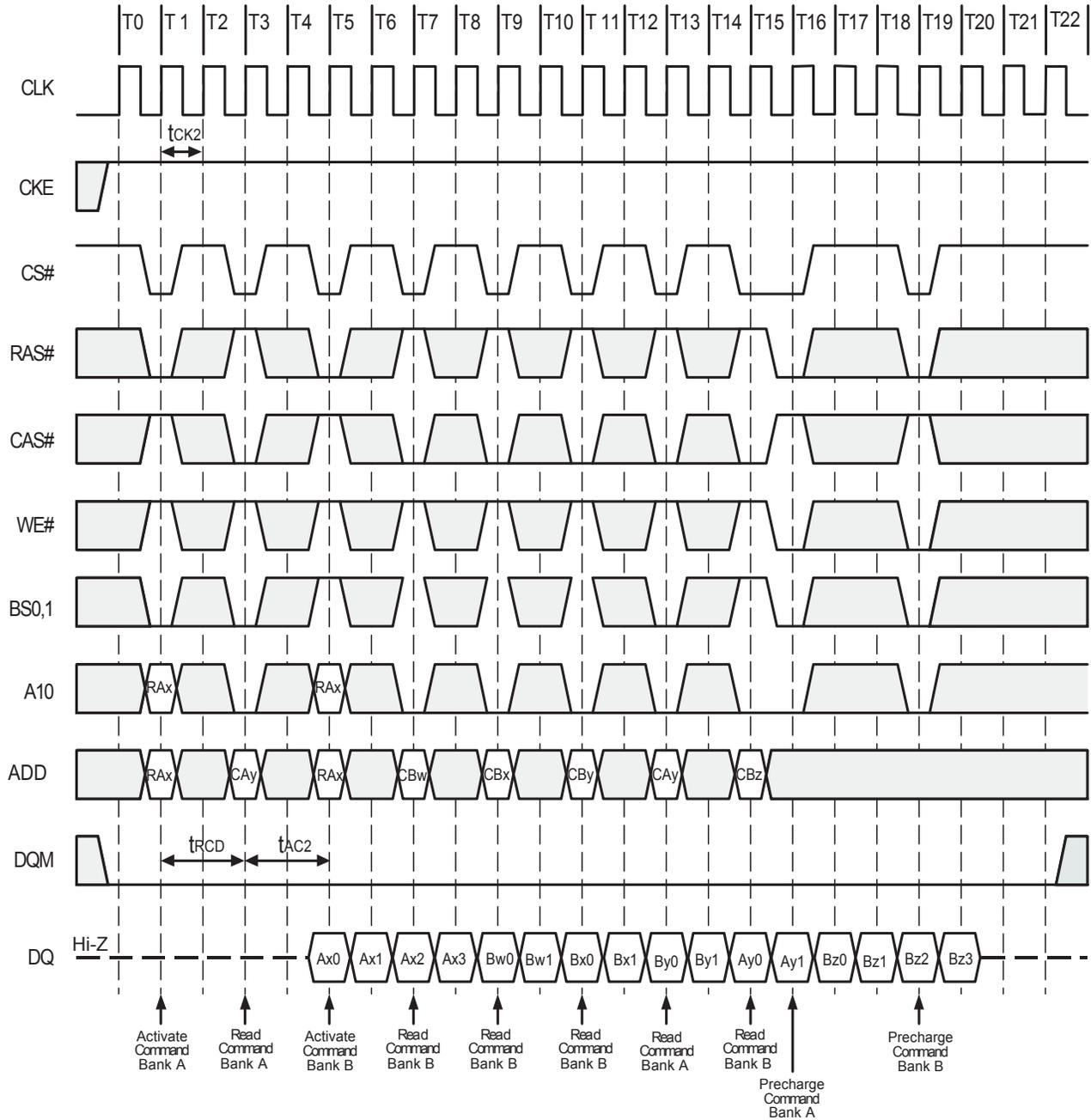
Interleaved Column Read Cycle (Burst Length=4,CAS#Latency=3)
