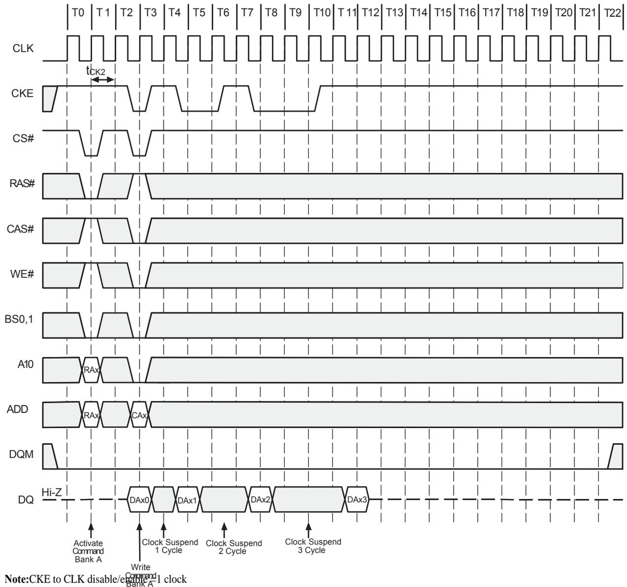
**Clock Suspension During Burst Write (Using CKE) (Burst Length=4,CAS#Latency=3)**
