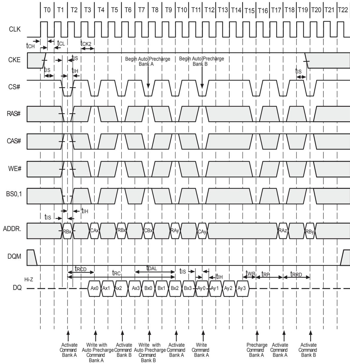
AC Parameters for Read Timing (Burst Length=2,CAS#Latency=2)
