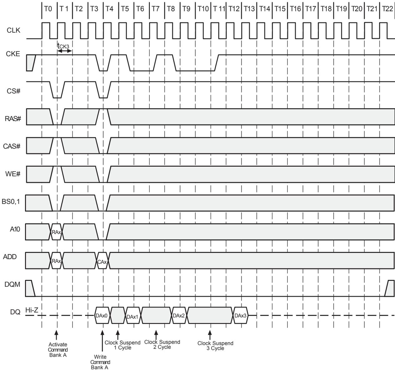
Power Down Mode and Clock Mask (Burst Length=4, CAS#Latency=2)
