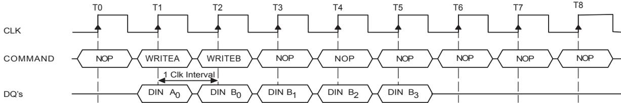
**Write Interrupted by a Write (Burst Length =4,CAS#Latency =2,3)**
