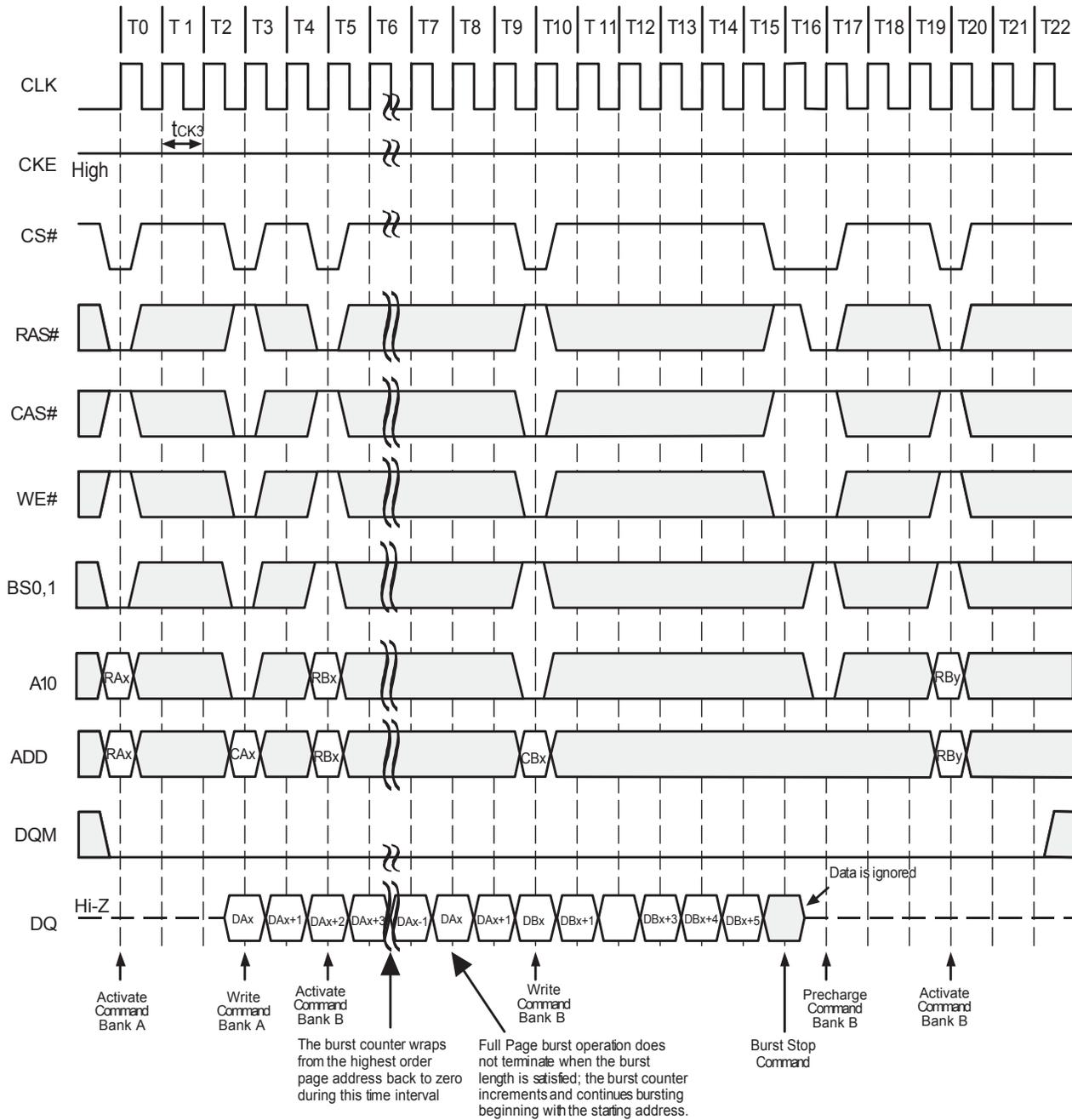
Byte Write Operation (Burst Length=4,CAS#Latency=2)
