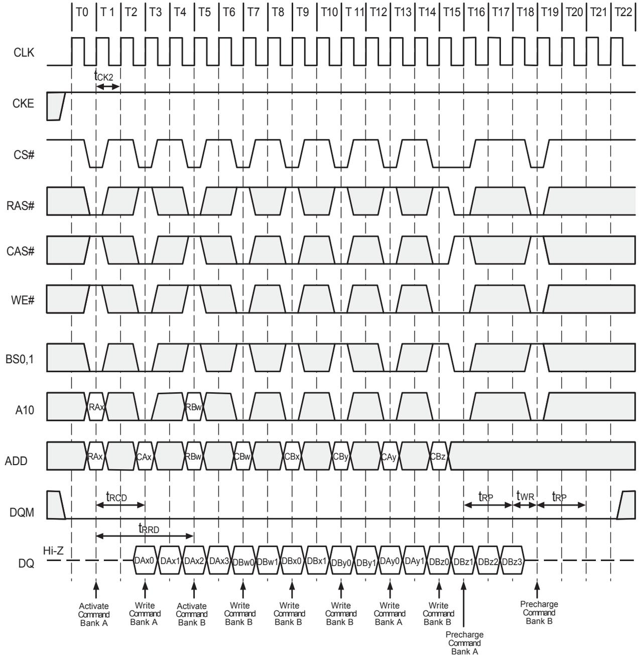
**Interleaved Column Write Cycle (Burst Length=4,CAS#Latency=3)**
