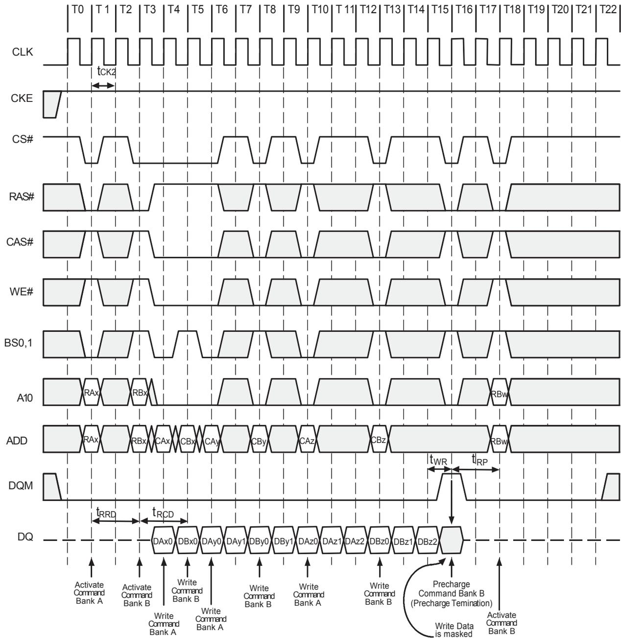
Precharge Termination of a Burst (Burst Length=8 or Full Page,CAS#Latency=2)
