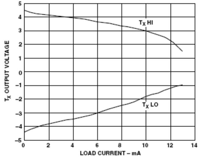
Figure 8. Transmitter Output Voltage vs. Load Current
