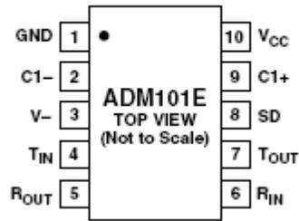
Figure 2. Pin Configuration
