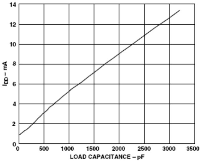
Figure 4. I<sub>DD</sub> vs. Load Capacitance at 460 kbps
