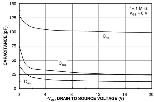
Figure 8. Capacitance Characteristics.
