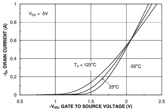
Figure 5. Transfer Characteristics.
