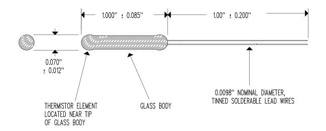
RESISTANCE @  $+25^{\circ}C$  = 10,000  $\Omega$  ± 5% RESISTANCE/TEMPERATURE CURVE = "J" BETA " $\beta$ " (+25 TO +85°C) = 3,977°K NOMINAL TEMPERATURE COEFFICIENT @  $+25^{\circ}C$  = -4.4%C NOMINAL TEMPERATURE RATING = -50 TO  $+300^{\circ}C$
