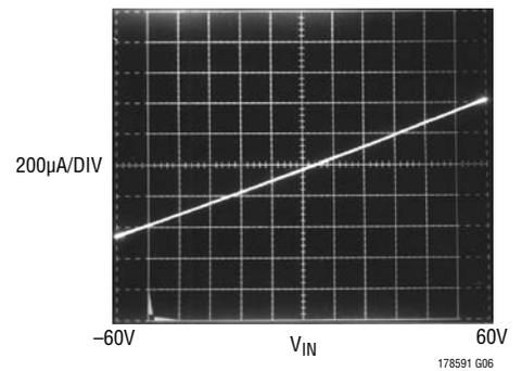
**LT1785 Input Characteristics Pins A or B; DE = RE = 0V**
