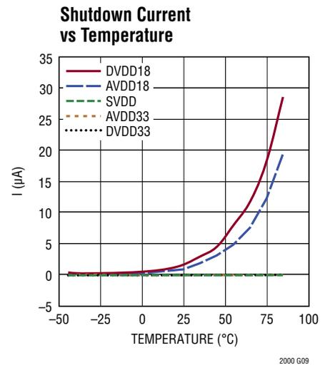
**TYPICAL PERFORMANCE CHARACTERISTICS**  $I_{OUTFS} = 40mA$ ,  $T_A = 25^\circ C$ ,  $AV_{DD18} = DV_{DD18} = 1.8V$ ,  $AV_{DD33} = DV_{DD33} = 3.3V$ ,  $R_{LOAD} = 12.5\Omega$ ,  $LIN\_DIS = 0$ ,  $LIN\_GN = 75\%$  unless otherwise noted.
