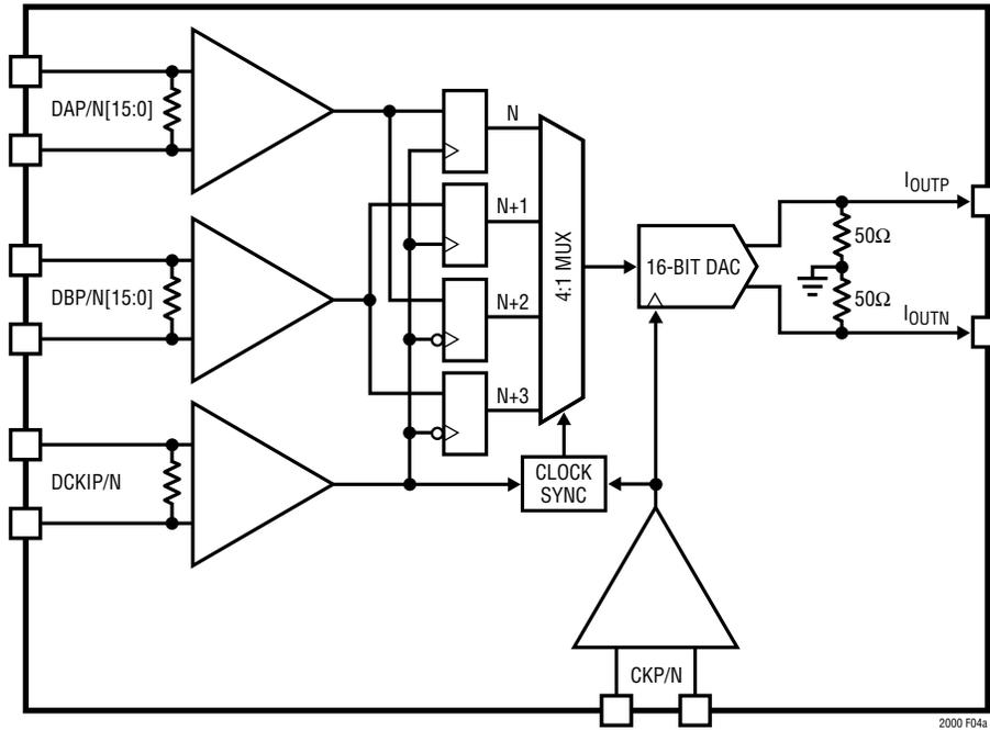
**Figure 4a. Simplified Block Diagram – Dual-Port Operation**
