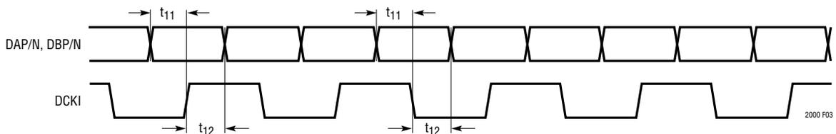
Figure 3. LVDS Interface Timing (DCKI\_Q = 1)
