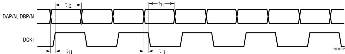
Figure 2. LVDS Interface Timing (DCKI\_Q = 0, DCK\_TADJ = 000)
