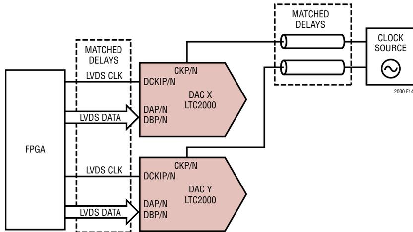
Figure 14. System with Multiple LTC2000 DACs Synchronized
