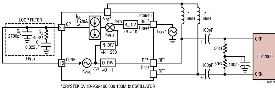
**Figure 13. DAC Sample Clock Generation with the LTC6946**
