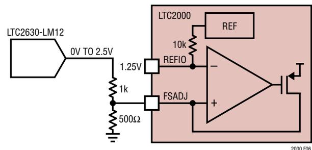
**Figure 6. LTC2000 Full-Scale Adjust from 20mA to 60mA**
