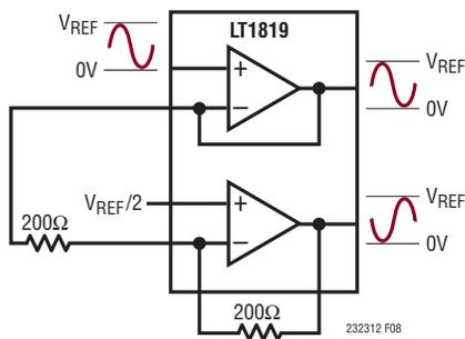
Figure 8. Single-Ended to Differential Driver
