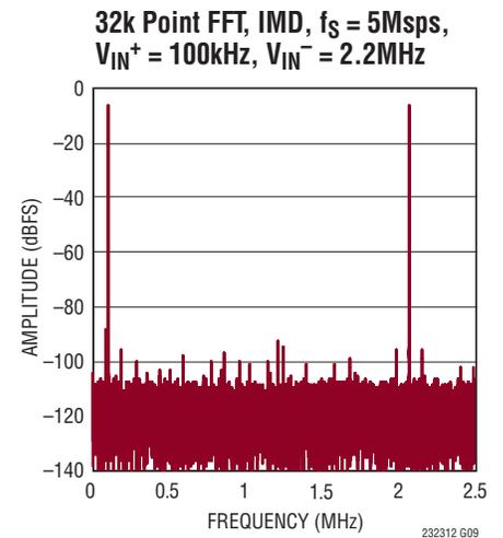
**TYPICAL PERFORMANCE CHARACTERISTICS**  $T_A = 25^\circ\text{C}$ ,  $V_{DD} = 5\text{V}$ ,  $OV_{DD} = 2.5\text{V}$ ,  $REF_{OUT1,2} = 4.096\text{V}$ ,  $f_{SAMPL} = 5\text{MSPS}$ , unless otherwise noted. (Note 16)
