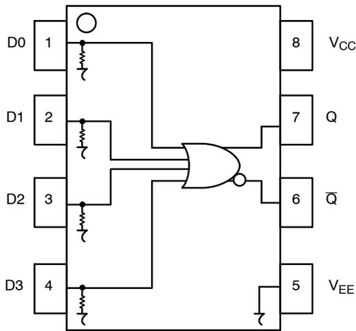
**Figure 1. 8-Lead Pinout (Top View) and Logic Diagram**
