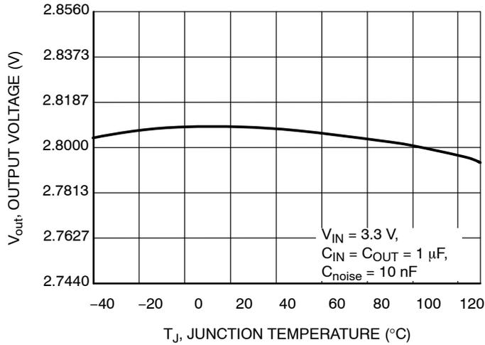
**Figure 4. Output Voltage vs. Junction Temperature,  $V_{OUT} = 2.8$  V**
