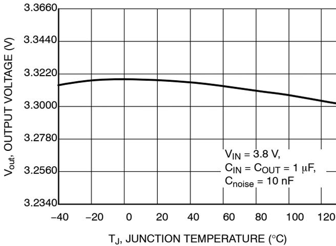
**Figure 6. Output Voltage vs. Junction Temperature,  $V_{OUT} = 3.3 V$**
