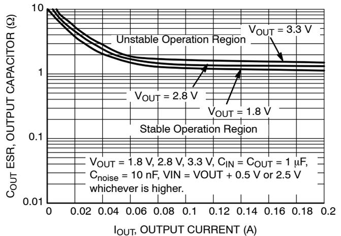
Figure 56. Output Capacitor ESR vs. Output Current
