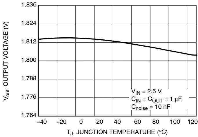
**Figure 3. Output Voltage vs. Junction Temperature,  $V_{OUT} = 1.8$  V**
