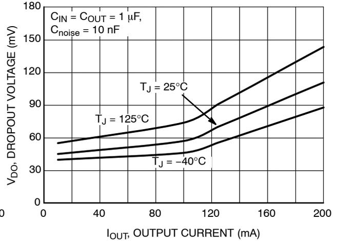
**Figure 9. Dropout Voltage vs. Output Current,  $V_{OUT} = 3.3 V$**
