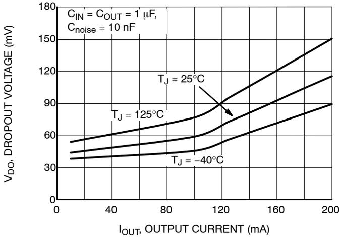
**Figure 8. Dropout Voltage vs. Output Current,  $V_{OUT} = 3.0 V$**
