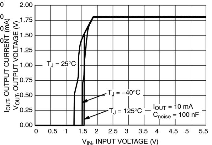
Figure 44. Output Voltage vs. Input Voltage,
