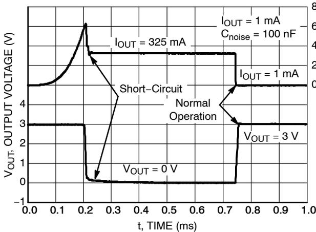
Figure 41. Short-Circuit Protection,
