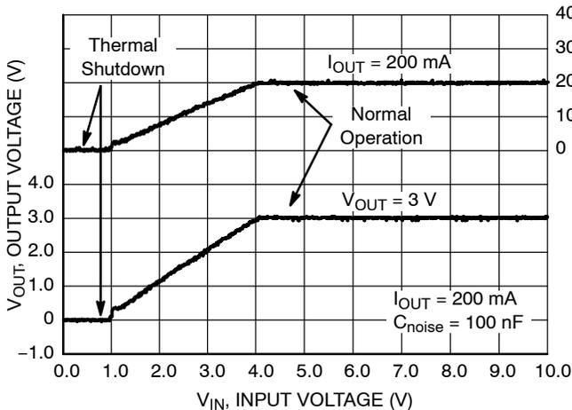
Figure 43. Thermal Shutdown Protection
