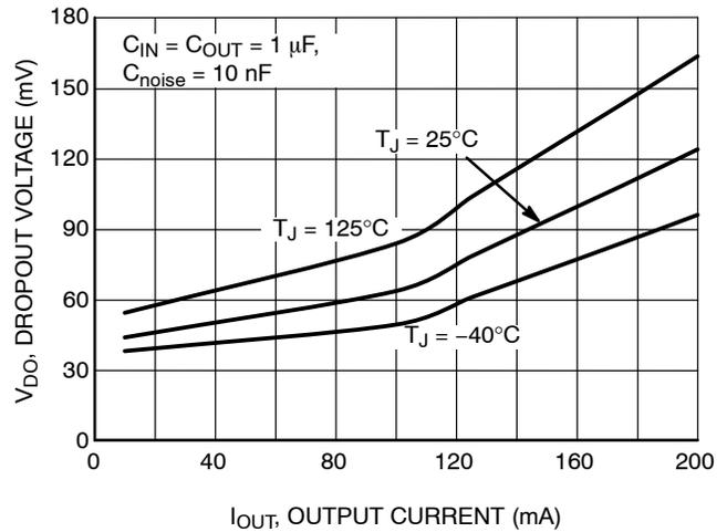
**Figure 7. Dropout Voltage vs. Output Current,  $V_{OUT} = 2.8 V$**
