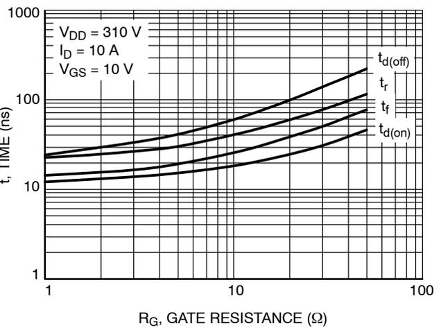
**Figure 10. Resistive Switching Time Variation vs. Gate Resistance**
