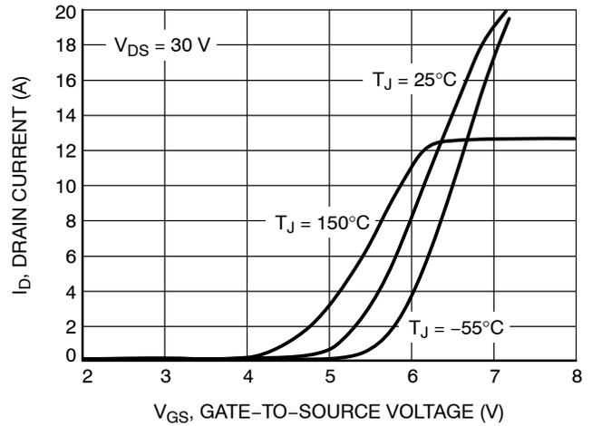
**Figure 2. Transfer Characteristics**
