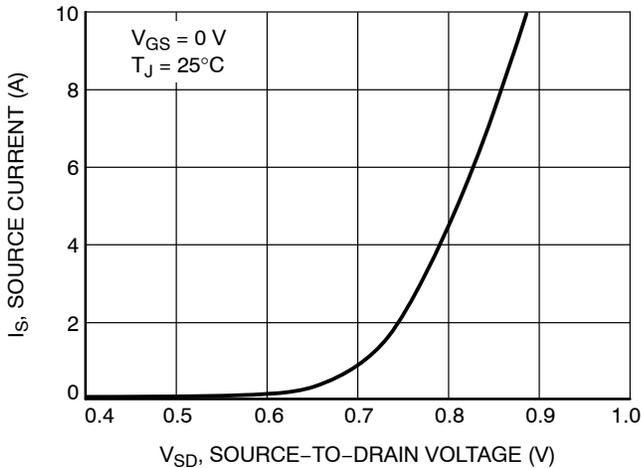
**Figure 11. Diode Source Current vs. Forward Voltage**
