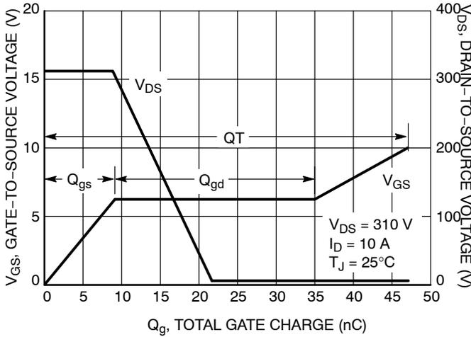
**Figure 9. Gate-to-Source and Drain-to-Source Voltage vs. Total Charge**
