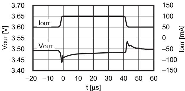
3. Transient response characteristics of ON / OFF pin (Ta = +25°C)
