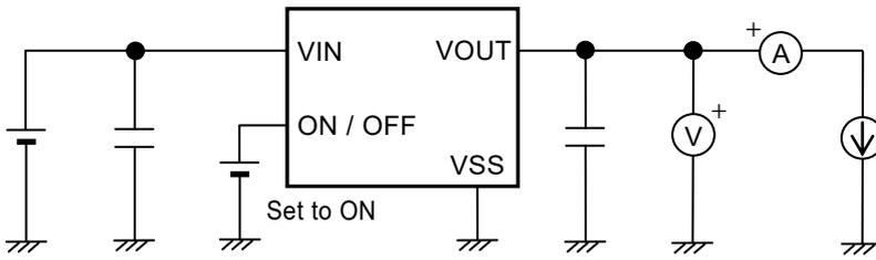
Figure 10 Test Circuit 1
