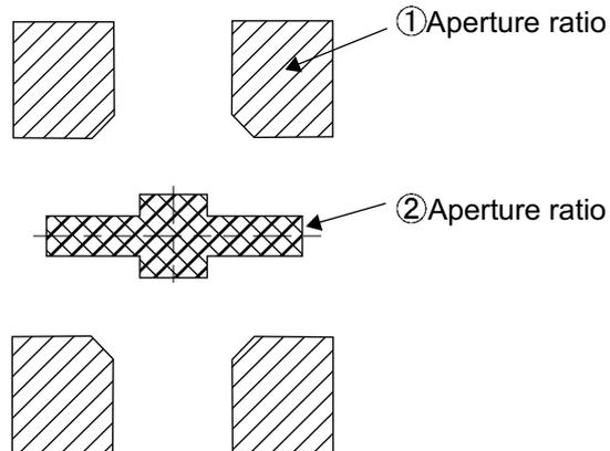
Caution ① Mask aperture ratio of the lead mounting part is 100%.
