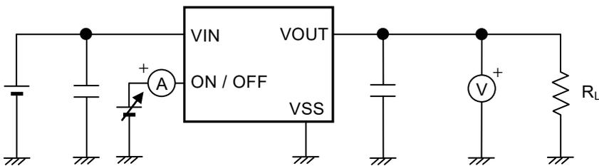
Figure 13 Test Circuit 4
