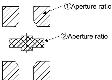
Caution ① Mask aperture ratio of the lead mounting part is 100%.
