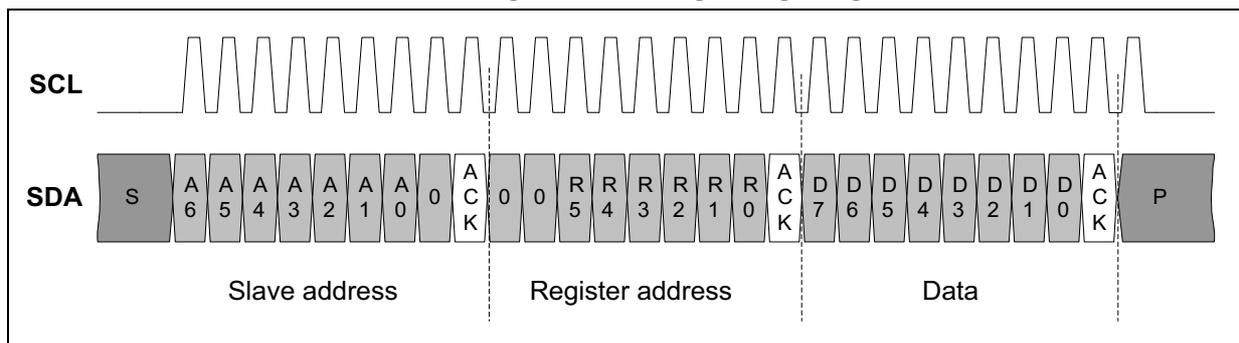
**Figure 21. Writing register data with auto-incrementing address**
