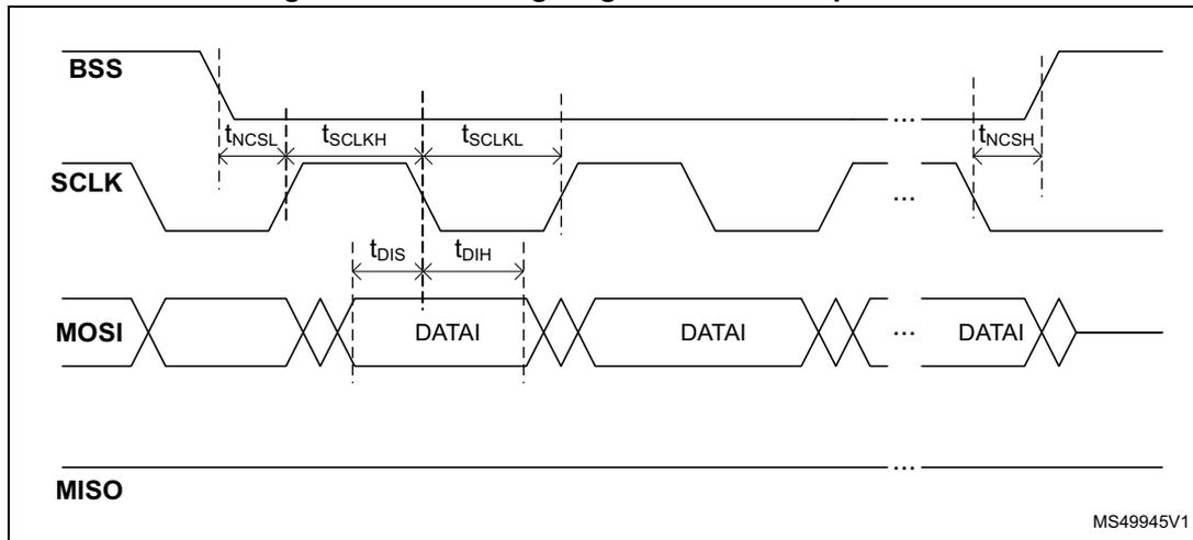
Figure 31. SPI timing diagram - Read operation
