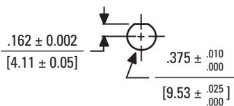
Note: Tolerance  $\pm .005$  [.13] unless noted angles:  $\pm 5^\circ$ . Dimensions in Brackets [ ] are millimeters.
