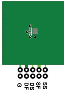
53  $^\circ\text{C}/\text{W}$  when mounted on a 1 in<sup>2</sup> pad of 2 oz copper
