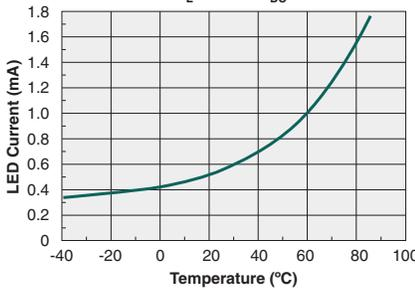
Typical  $I_F$  for Switch Dropout vs. Temperature
