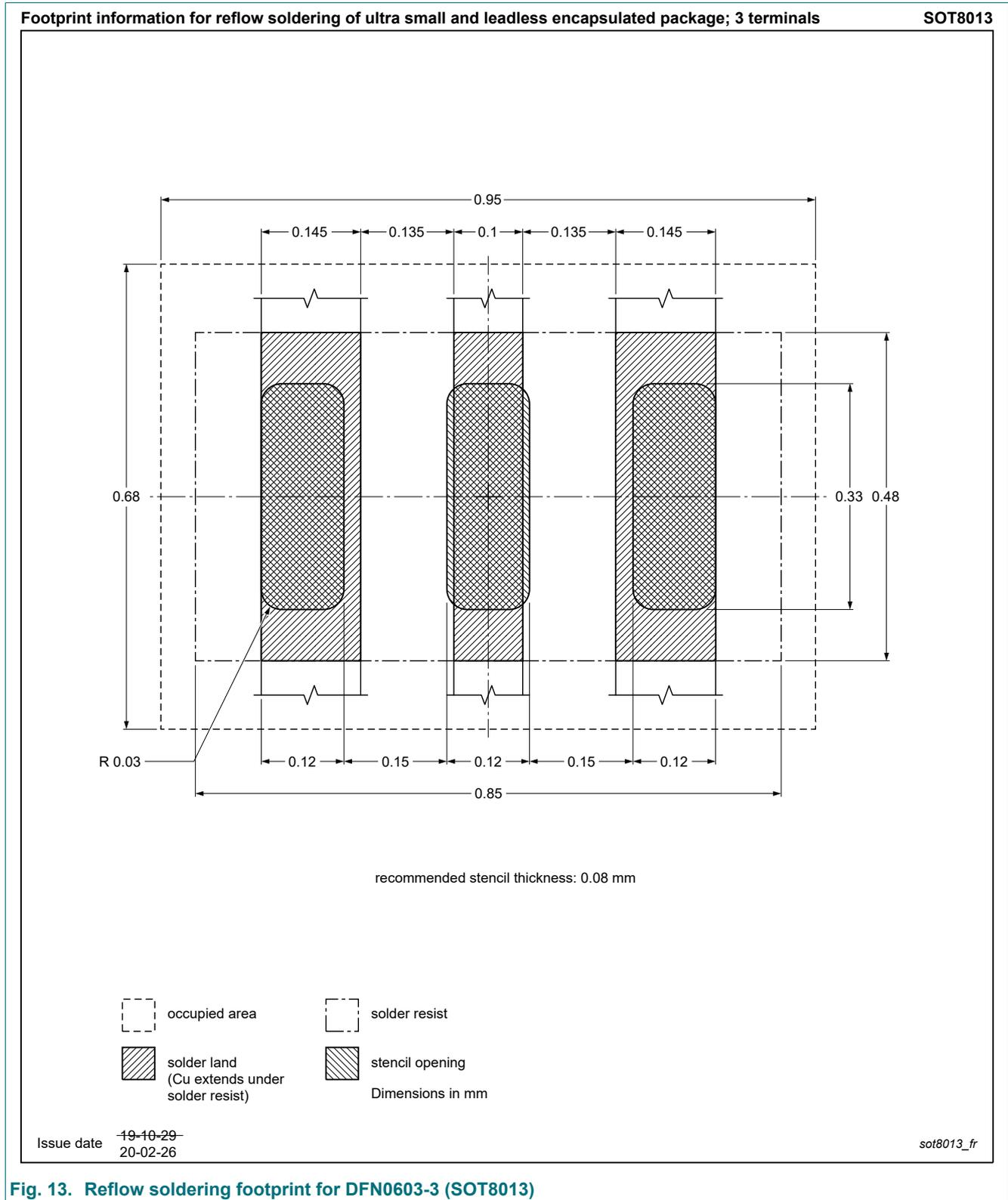
Fig. 13. Reflow soldering footprint for DFN0603-3 (SOT8013)
