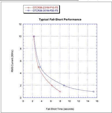
Note: Both electrodes simultaneously powered, each with the AC current value in the graph
