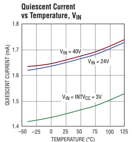
**TYPICAL PERFORMANCE CHARACTERISTICS**  $T_A \approx T_J = 25^\circ\text{C}$ , unless otherwise noted.
