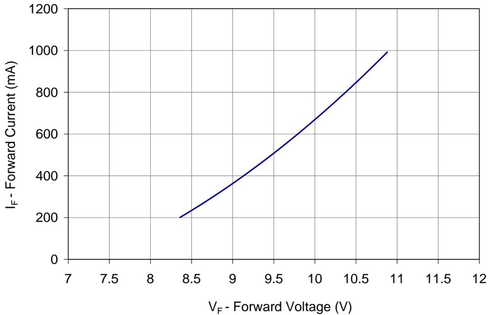
Figure 9: Typical forward current vs. forward voltage @ T<sub>c</sub> = 25°C.
