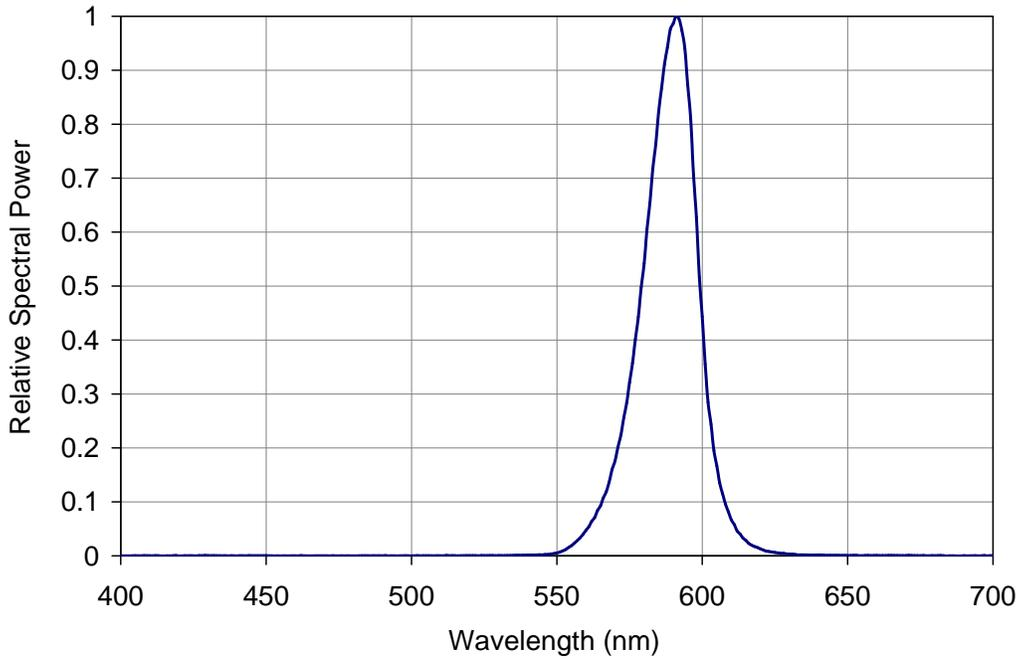
Figure 5: Relative spectral power vs. wavelength @  $T_c = 25^\circ\text{C}$ .
